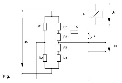
The connection of resistor R7 will always result in a defined unbalancing of the zero point (diagonal voltage) of the Wheatstone Bridge.
