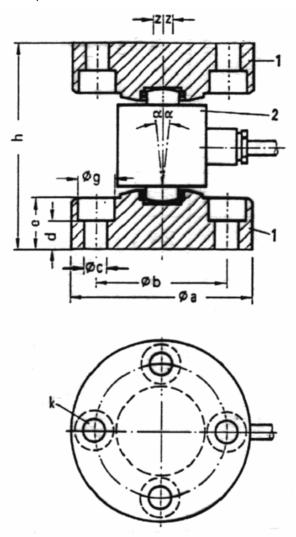
Horizontal deflections (z) of the load bearer cause an inclination (  $\alpha$ ) of the force transducer. As a result the build-in height simultaneously increases. During installation,  $\alpha$  can be utilised up to 6°.
