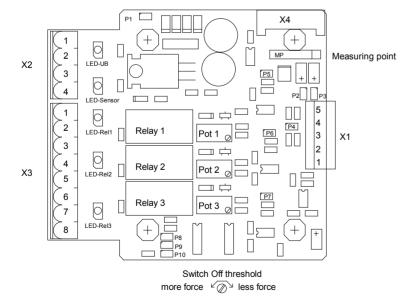
AC / DC P1 P2 Filter РЗ Filter P4 1-9mA / 4-20mA hysteresis Rel 1 P5 P6 hysteresis Rel 2 P7 hysteresis Rel 3 P8 Rel 1 closing / opening P9 Rel 2 closing / opening P10 Rel 3 closing / opening
