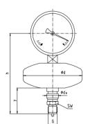
Open process connection DN 15 ... 50, PN 6 / 40 Connection dimensions to DIN 2501
